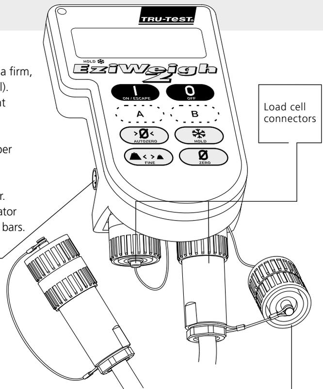
Dust caps screw together to keep out dirt and moisture when cables are connected to indicator. Screw back on indicator/cables when cables removed.
