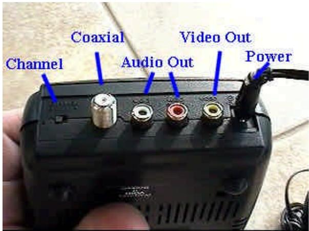
You can hook the receiver up to your TV with either the RCA cables (the three colored cables) or the coaxial cable (thick black cable). They are both offered as an option. Do not plug in both as it will not work.
