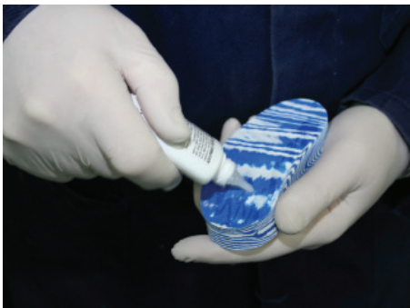
Fig 3. Apply glue sparingly to the Walkease Block
