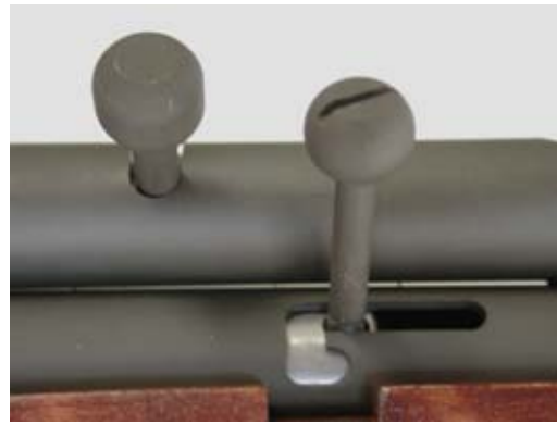
Fig. 3 Cocking Knob in High Power Position
