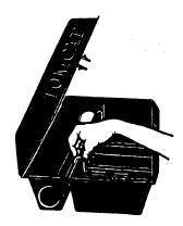
Insert the hooked end of the rod into the hole on top edge of the baffling and snap down to secure.
