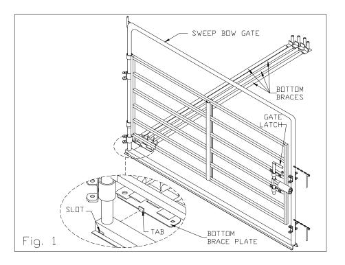
NOTE: The slots on the Bow Gate are for assembling the sweep tub on either side of the gate. When assembling the tub on the opposite side of the Bow Gate as shown, you will need to move the Gate Latch to the other side of the gate. You will also need to move the far left Bottom Brace to the open hole on the right side of the Brace Plate.
