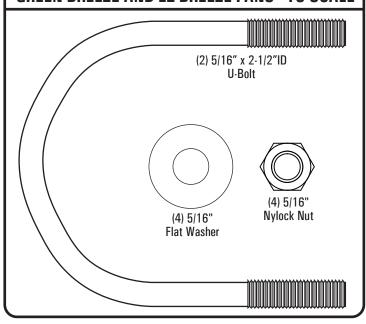
Using the installation hardware shown above you can mount the included bracket as shown below. Drawing "C" is acceptable without contradicting the space requirement mentioned in step 1 on page 2 as long as there is nothing behind the pipe to impede air flow. Use (2) 5/16" flat washers and (2) 5/16" nylock nuts for each u-bolt used, assembled as shown below in drawing A.
