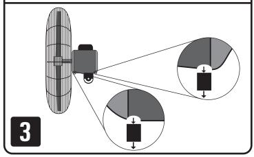
Attach fan to bracket. Insert bracket flag in between the motor flags and secure using the center holes on the motor flags with (1)  $3/8" \times 1.1/4$  hex bolt, (2) 3/8" washers and (1) 3/8" nylock nut as shown in step 4a. Using the crescent openings on the motor flags, install the (1)  $1/4" \times 1$ - hex bolt, (2) 1/4" washers and (1) 1/4" nylock nut as shown in step 4b. Adjust the fan to the desired angle and tighten hardware to secure fan angle.
