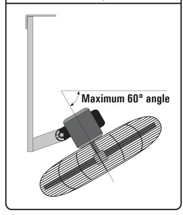
Do NOT operate the fan with the motor mounted in a vertical orientation, or at any angle larger than  $60^{\rm o}$  from horizontal as shown above. Mounting this way will void the warranty.
