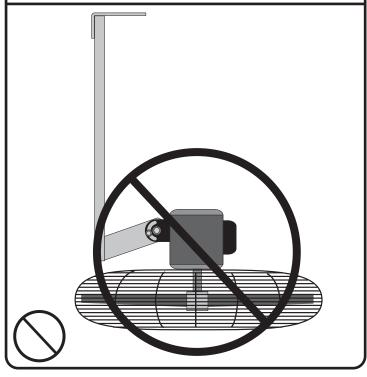
Do NOT mount fan with capacitor on the bottom. This can cause moisture to build up in the capacitor cap and short out the capacitor. Mounting the fan this way will void the warranty.
