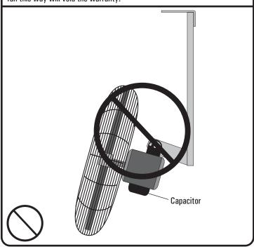
Do NOT mount bracket horizontally. The included bracket was not designed to be mounted this way and cannot withstand the structural stress caused by the weight and movement of the fan. Mounting the bracket and fan this way will void the warranty.
