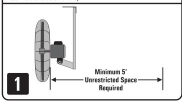
If mounting bracket to structure, verify anchor points are strong enough for added weight of bracket and fan. Attach top of bracket to structure with (4) washers and (4) screws or bolts with nylock nuts (not provided) suitable for your structure. DO NOT attach bracket to or against wall as this will not give motor enough unrestricted air flow. (For pipe mount instructions see page 4.)
