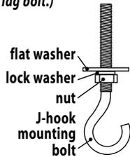
Using a drill and drill bit, drill a hole thru joist. Insert J-hook mounting bolt with assembled hardware into hole and secure with flat washer, lock washer and nut as shown below.
