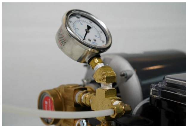
Figure 3 – Pressure Gauge Mounted Into Brass Cross Assembly
