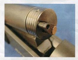
Once you have rotated the Blank Adaptor push in on the blank adaptor and the power load case can easily be removed from the blank adaptor chamber.
