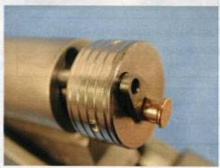
Release the adaptor and remove power load from adaptor. Extractor will return to position in adaptor.
