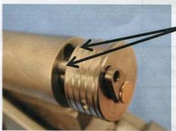
Pull back on blank adaptor until the pin is out of the slot in the barrel and rotate adaptor counterclockwise to 10:00 or until pin is free of slot in barrel.
