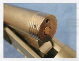
Depress Breach lever to expose Blank Adaptor
